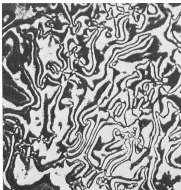
Figure 4. The schlieren texture (Lehmann 1904).
